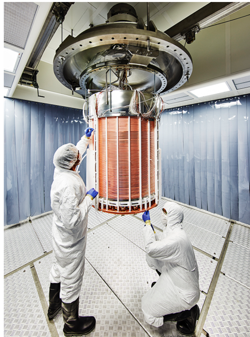
TPC installation underground
