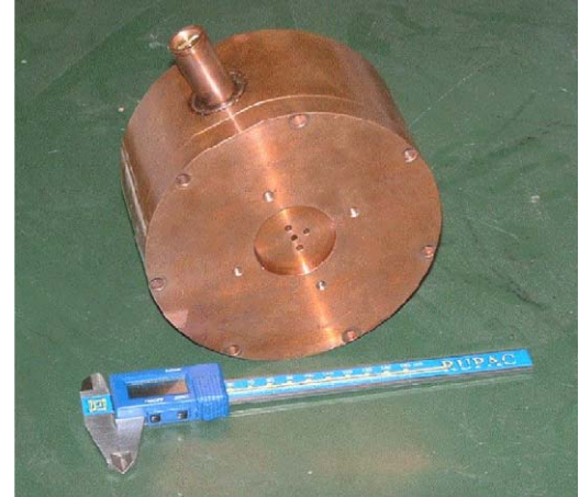
Fig. 26. Pillbox cavity used for calibration of perturbing objects.
