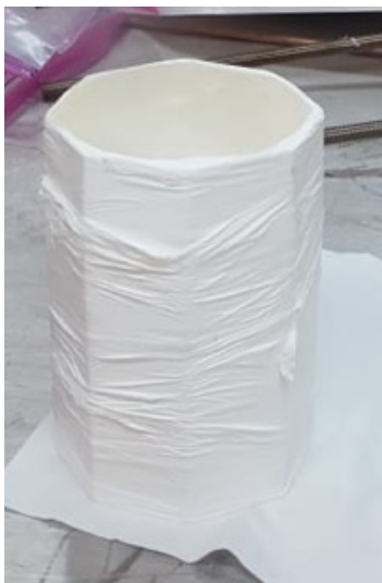
Crystal NaI-31, grown in a standard quartz crucible. Mass: 3.7 kg after polishing. Produced in June 2018.
