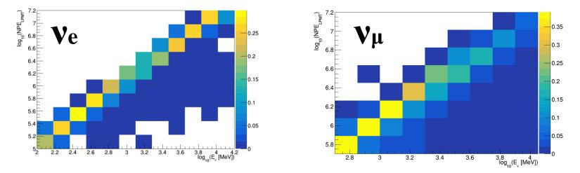
The inverse relationship allows to infer the neutrino energy spectrum from the detector observable distribution
