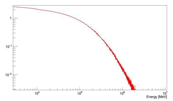
Sampling of the spectrum to evaluate the background inside JUNO, in terms of PE  $\rightarrow$  energy and inclination
