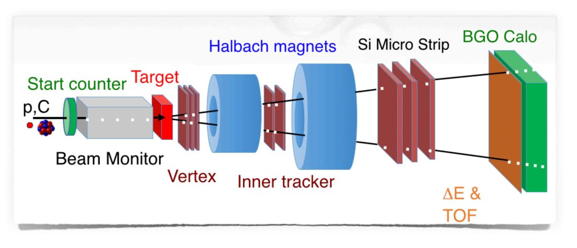
\* Structure similar to other detectors. Main work on Geometry (MC) and Mapping (data)
