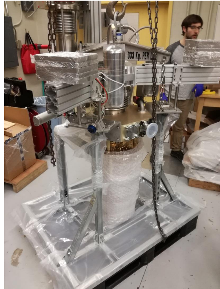
Alignment system designed and tested for secure cryostat lifting
