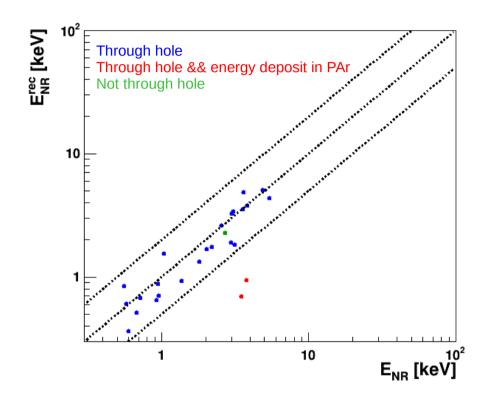
1 golden event out 26 is due to a neutron that scatter slightly in the Shield. Collimation is working.
