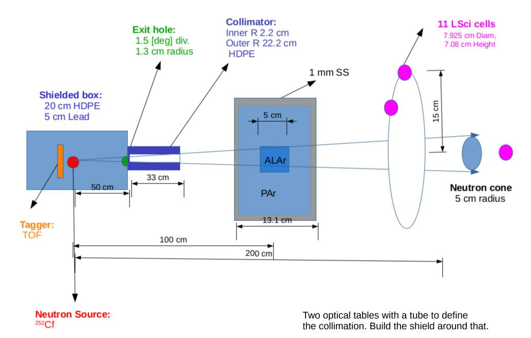
A lead cap on the collimator cylinder might be appropriate. Needs to be studied.
