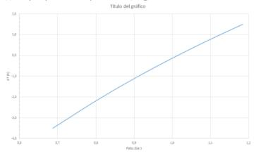
The temperature difference of 2,7 mK correspond to a differential pressure of roughly 0,3 mbar that is negligible.
