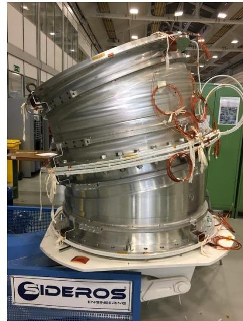
The second unit (2 modules) is now at Fermilab under preparation for the cryogenic test.
