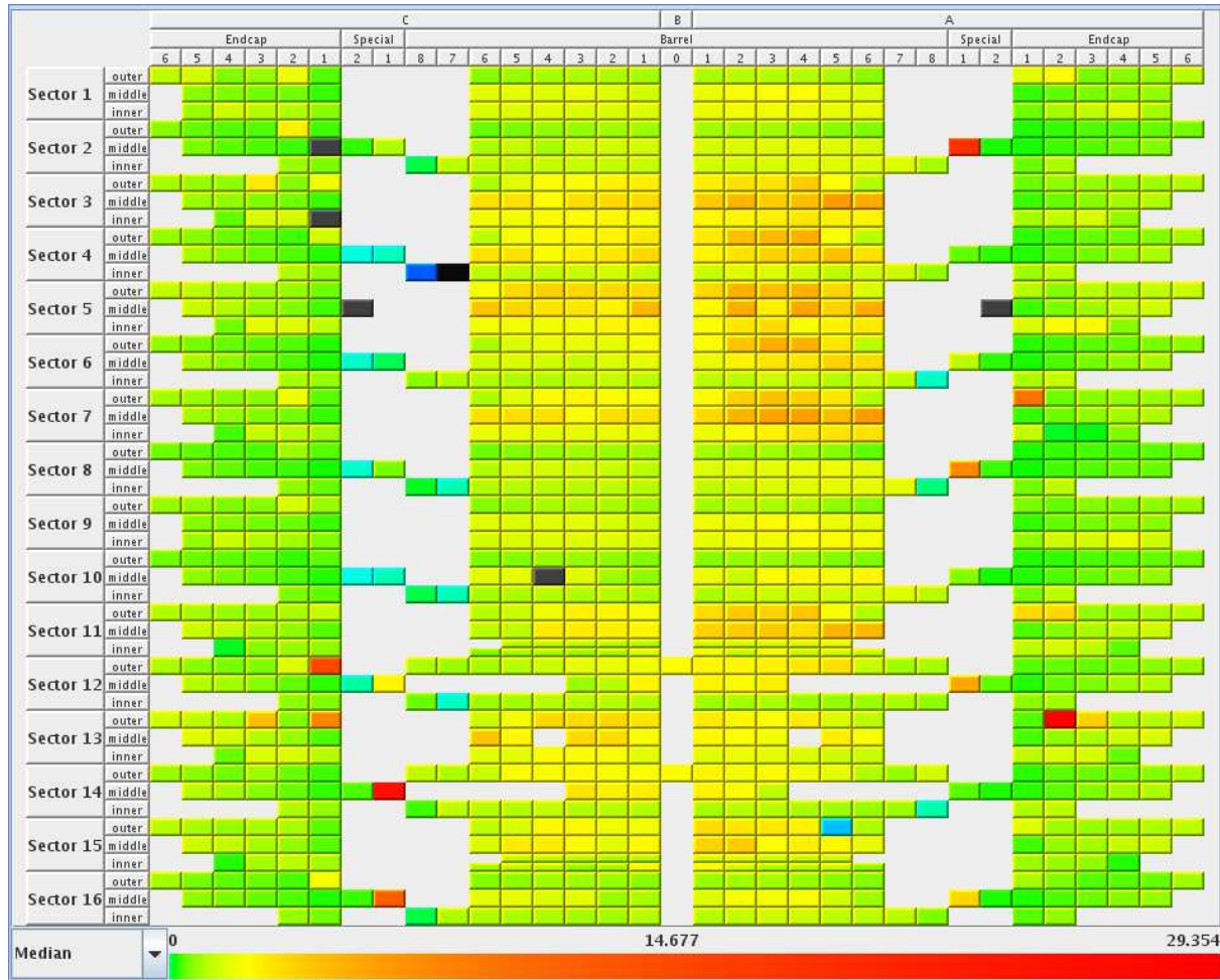
Figure 1: Screen-shot of a monitoring application displaying the MDT hit occupancy for all ATLAS MDT chambers. Each chamber is represented by a small box. The color of the box is related to the median number of raw hits per tube in that MDT chamber in logarithmic scale. The boxes are arranged in a grid, in which a column represents a slice perpendicular to the ATLAS beam axis. The rows are grouped into the sixteen sectors of the ATLAS MDT system. Within each sector chambers of the Outer, Middle and Inner ring of chambers are displayed.
