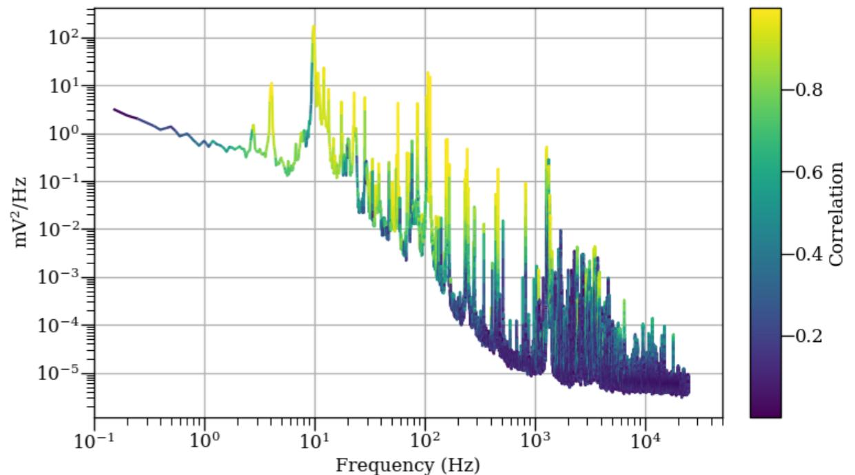
Accelerometer-flux noise correlation
