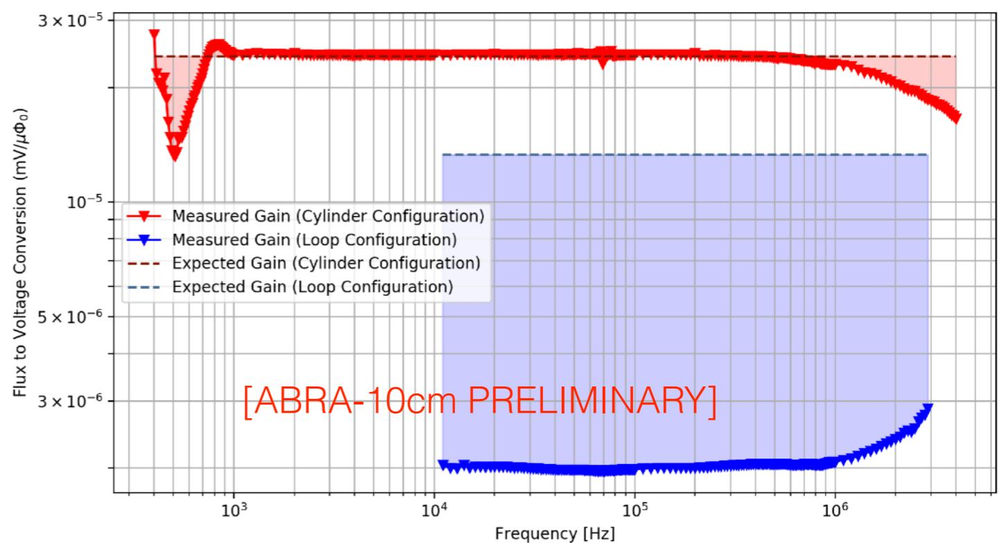
Incorporating active feedback to reduce noise below 1 kHz
