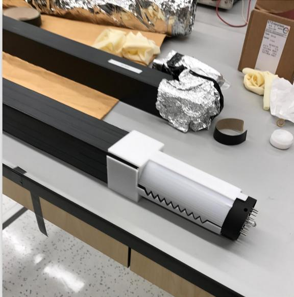
Bars wrapped in layers of reflective and light blocking materials (including tyvek, tinfoil, electrical tape)
