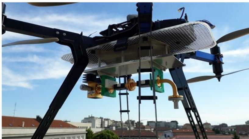
Payload mounted on the UAV
