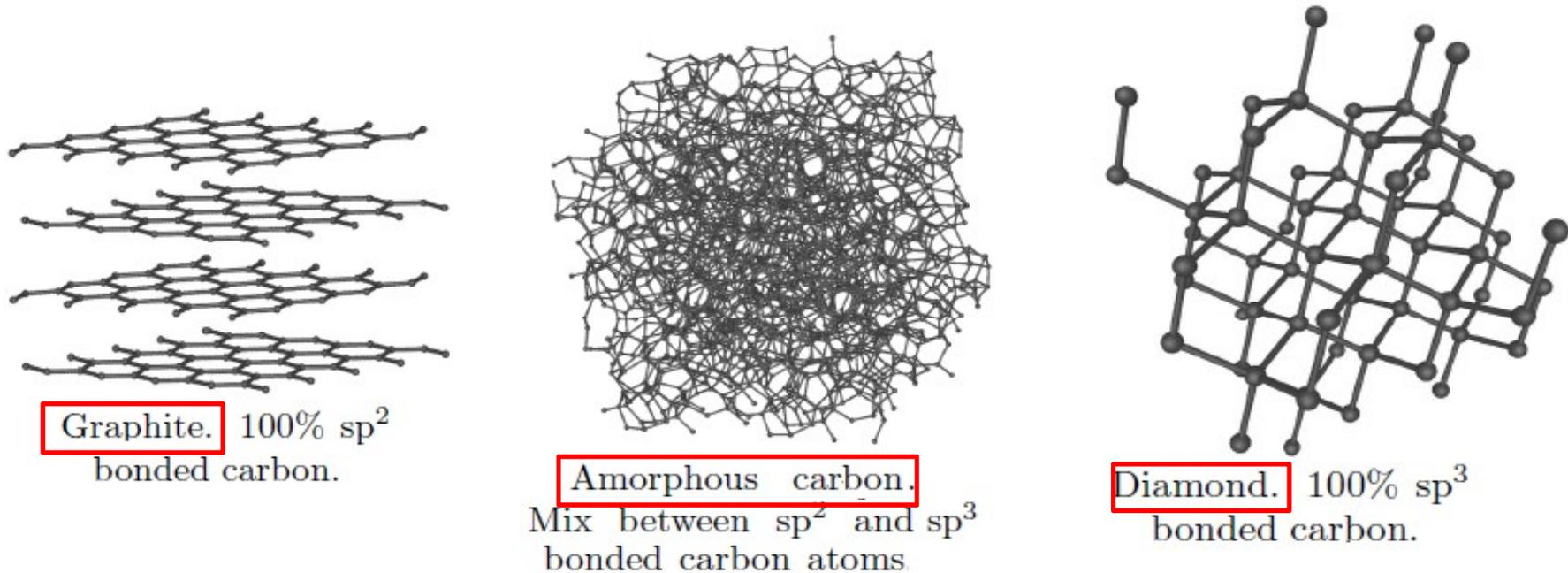
This bond configuration is such to confer to DLC particular properties intermediate between that ones of diamond and graphite which can be modulated by the  $sp^3/sp^2$  fraction.
