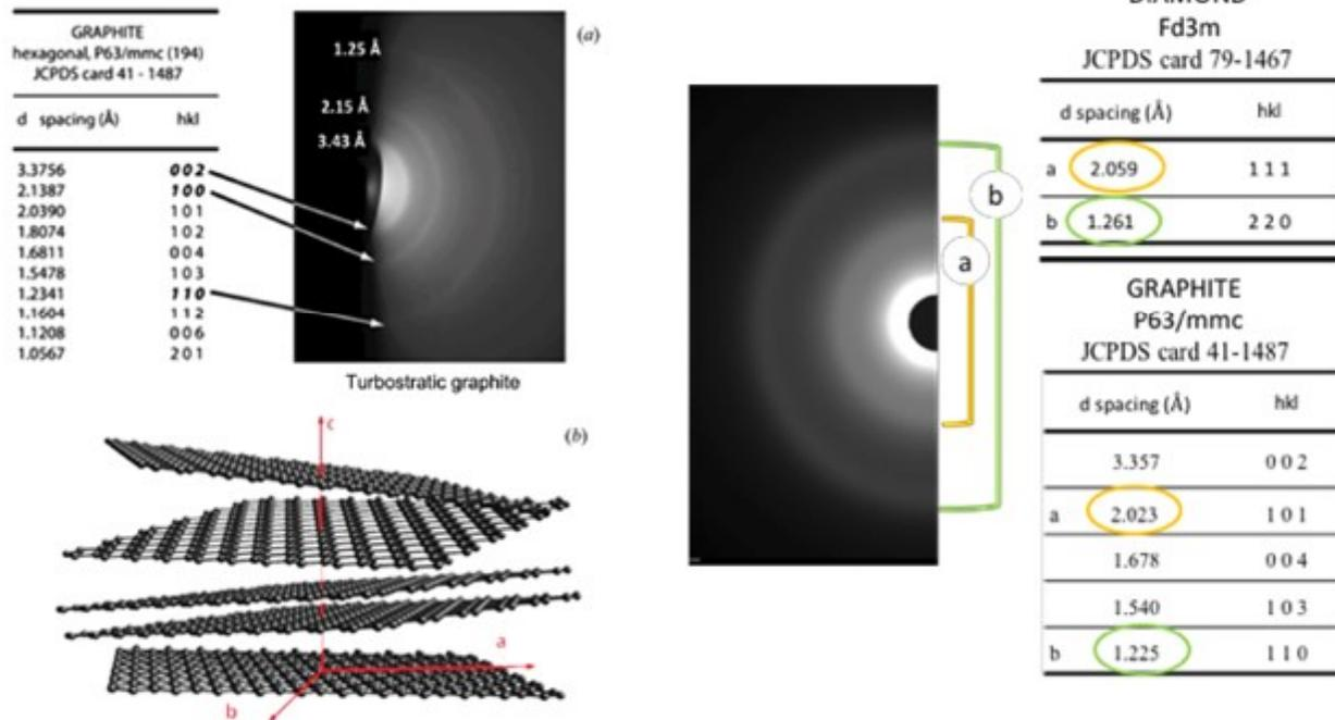
Two rings are clearly visible which are compatible with both the diffraction maxima 111 and 220 of the diamond, and with the diffraction maxima 101 and 110 of the graphite. This can be interpreted as an overlapping of nano-graphene (missing the ring corresponding to the planes 002 of the graphite) and nanodiamond.
