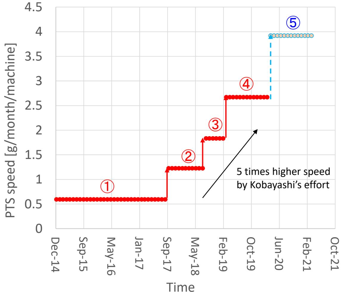
① : 1st PTS machine : no special techniques for high scanning speed
