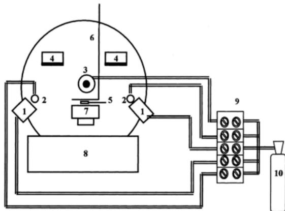
**FIGURE 1** Schematic representation of the dual ion-beam sputtering deposition system used: (1) sputtering ion-beam sources, (2) plasma bridge neutralizers, (3) assistance ion-beam source, (4) targets, (5) quartz microbalance, (6) shutter, (7) substrate holder, (8) turbomolecular pump, (9) flow control unit, (10) argon supply
