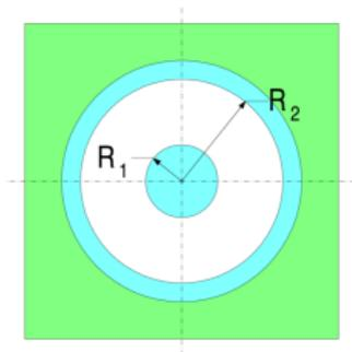
$$\rho_S = R_S \frac{2\pi}{\ln \frac{R_2}{R_1}}$$
