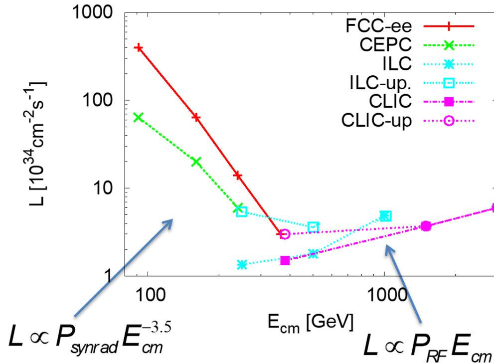
Use a linac to avoid synchrotron radiation
