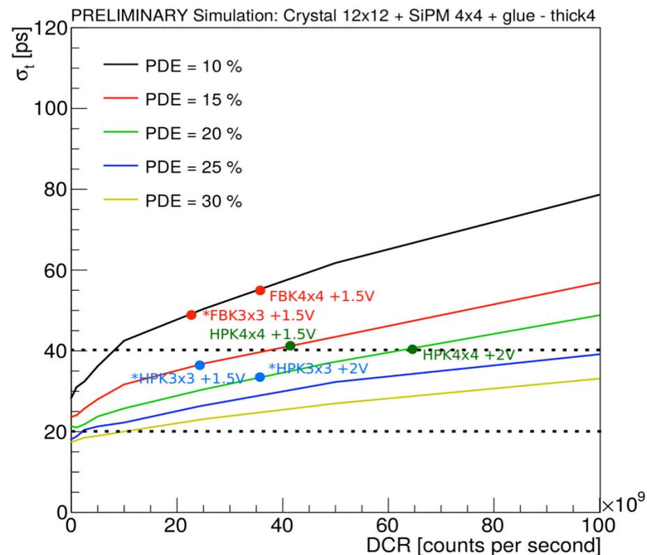
▶ To optimize: reflective wrappings, SiPMs size / layout, thicker tiles, ...
