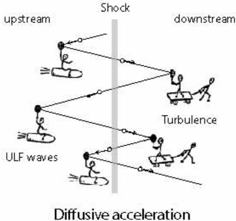
$$\langle \frac{\Delta E}{E} \rangle = \frac{4}{3} \frac{v_1 - v_2}{c}$$
