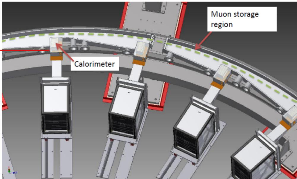
Individual positrons from muon decays are detected in 24 calorimeters;  $E$  and  $t$  extracted from waveforms. Each calo. segmented into  $6 \times 9$  channels: Each  $\text{PbF}_2$  crystal is read out by a Geiger-mode avalanche photodiode (SiPM).
