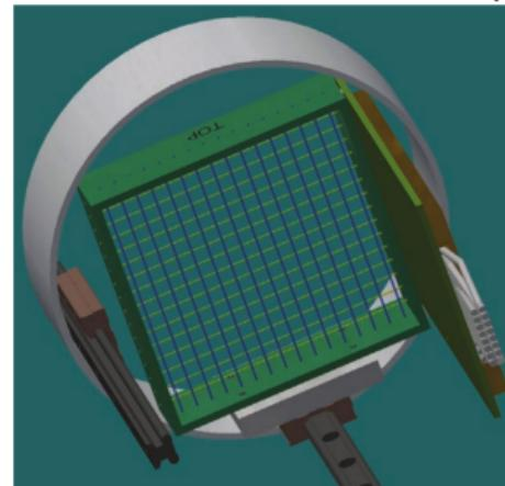
2 det's with 2 planes/each (scint-iber), upstream of inflector; 1 vertical plane (x) downstream of inflector (retracted during data taking):
