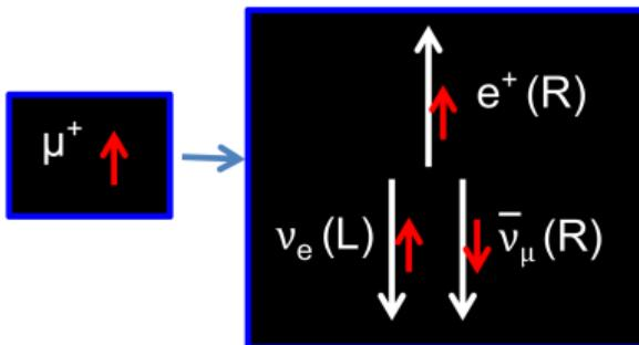
Positron direction follows muon spin
