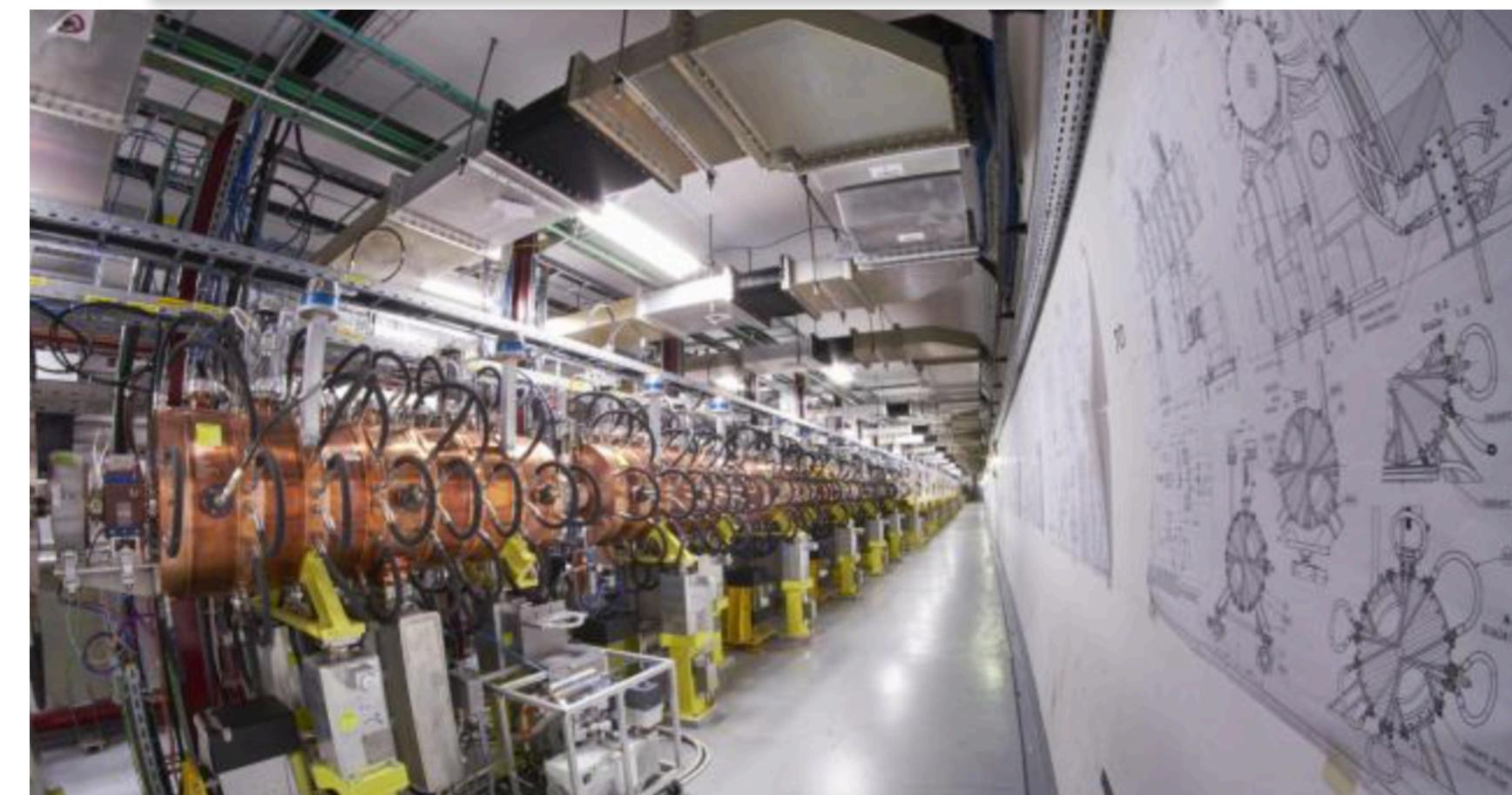
Will be accelerating negative Hydrogen ions. The electrons are stripped from the proton from the LINAC to the PS Booster (improves efficiency, intensity and quality).
