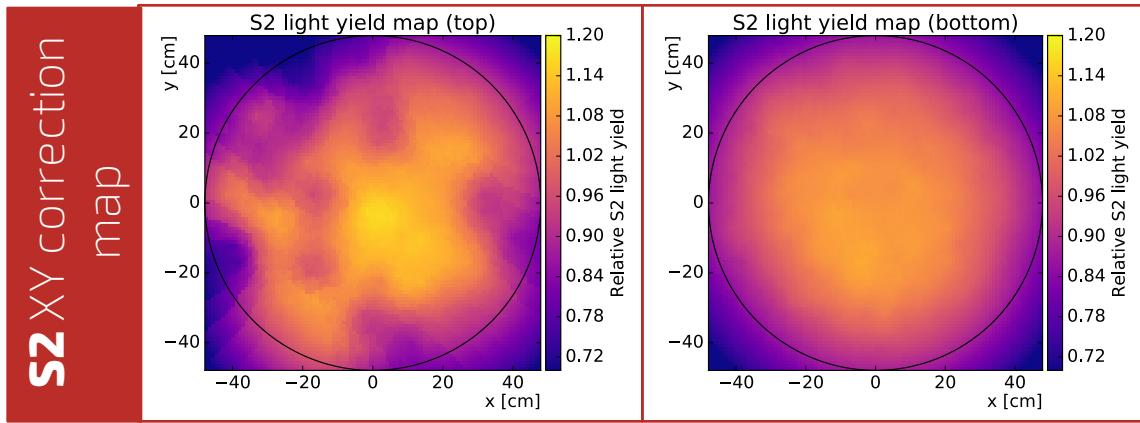
$^{83m}\text{Kr}$  source injected in LXe which uniformly distributes in the whole TPC volume → Ideal to understand spatial dependence of the light (S1) and charge (S2) signals.
