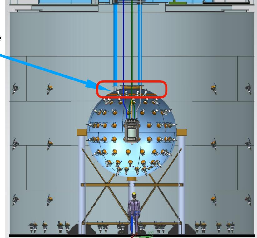
CTF Flange into the CRH to be removed
