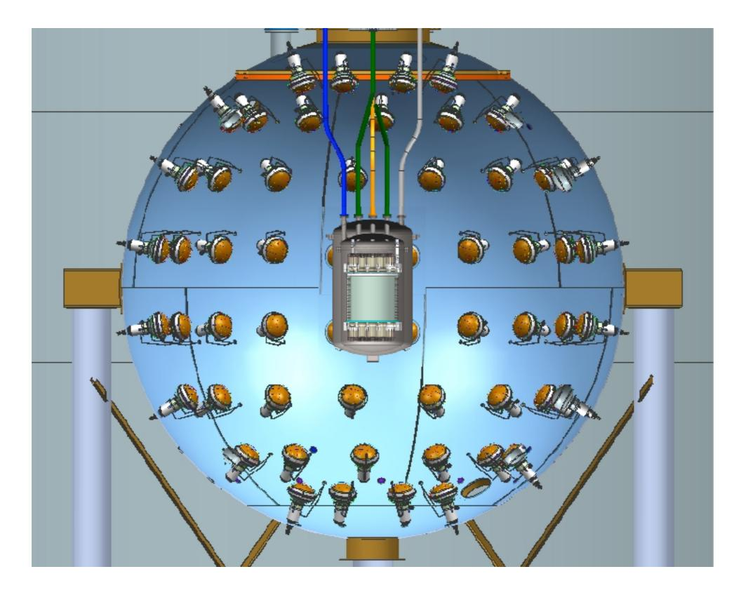
Liquid Argon TPC 153 kg <sup>39</sup>Ar-Depleted Underground Argon Target 4 m Diameter 30 Tonnes Liquid Scintillator Neutron Veto 10 m Height 11 m Diameter 1,000 Tonnes Water Cherenkov Muon Veto
