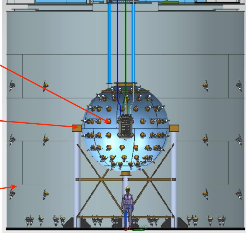
To insert the Proto into the LSV, we need to remove the upper dome
