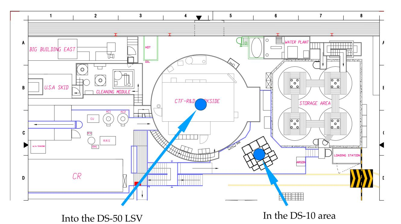
Note: Both the allocations are provided with electrical power, UPS, gas and liquid nitrogen. All the infrastructures used by DS-50 could be re-used....
