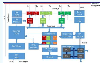
Qseven modules support different operating systems. Debian 7 version has been installed on the module. Collector processes, based on *libusb* library, continuously read USB FIFO using. The *Run Control* is based on the MIDAS data acquisition software developed at PSI and TRIUMF. The package includes a web interface.
