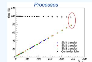
The Controller operates a real time tracking of the SM data transfer to optimize the overall performance. Duty cycle and toggle rate of all the *busies* are measured and attached to the data frame to be immediately correlated to the laser pulse pattern
