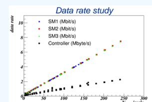
Linear behavior of the data transfer: SM and Controller measurements are carried out inside the Controller. The maximum value of slave data transfer is ~ 8 Mb/s. By design the peak value is about 9 Mb/s.
