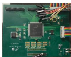
Various tests were performed on the nSYNC before the production phase. The test setup composed by a Logic Analyzer, a pattern generator (PGA), the I<sup>2</sup>C interface, the oscilloscope and the nSYNC test board, shown on the picture nearby.
