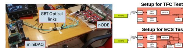
Each I<sup>2</sup>C bus tested performing 1024 read/write operations on each nSYNC and slave GBTx, with no errors. Tested the GPIO lines, in both I/O modes. ADC lines successfully used to monitor all power supply voltages. TFC commands continuously sent from miniDAQ to all nSYNCs for 2h: checked the number of sent/received commands and alignment of counters.
