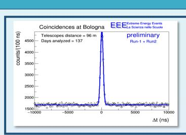
The detection of an EAS is achieved by measuring the coincidences in time recorded at different sites of the EEE Telescopes Array [3]
