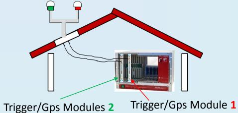
The difference between the signals from the reference module 1PPS<sub>ref</sub> and from the other modules 1PPS<sub>N</sub> was measured with an oscilloscope.
