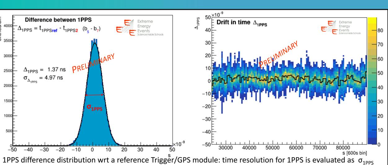
from a distribution gaussian fit, for module SN7, SN16 (using module SN5 as reference). Each distribution profile exhibits adequate stability in time.
