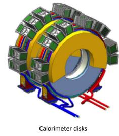
1 crystal coupled to 2 large ( $14 \times 20$  mm<sup>2</sup>) area UV-extended SiPM (total of 2696 electronic channels).
