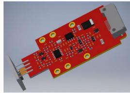
20 FE boards controlled by 1 mezzanine board in the DAQ crate: SiPM LV and HV distributed by an ARM controller.
