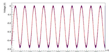
Analyzed more than 300 GB of data from neutron and TID tests, no evidence of bit flips or waveform shape variation.
