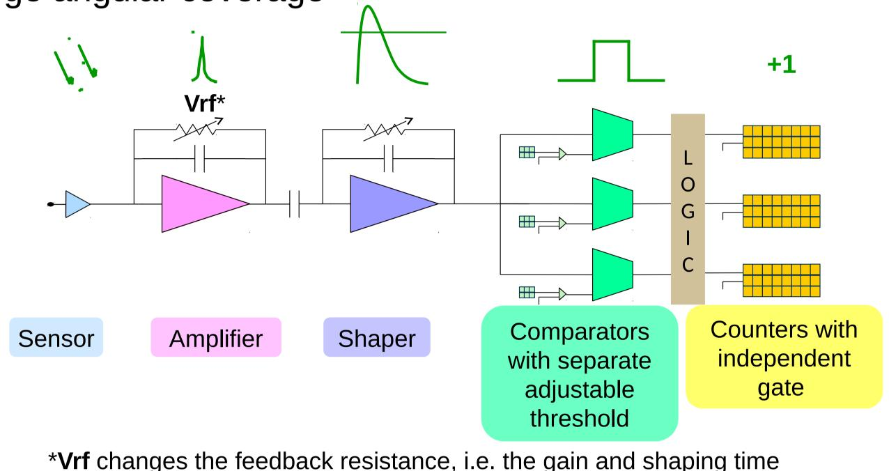
\*Vrf changes the feedback resistance, i.e. the gain and shaping time
