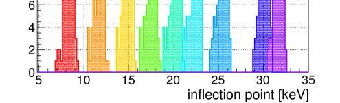
The threshold dispersion is given by the spread of the inflection points, i.e. the resulting thresholds, over all sensor-strips.
