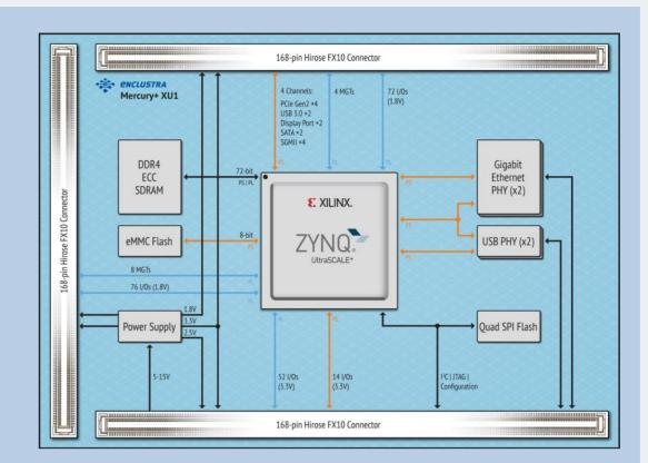
16nm FinFET+ FPGA fabric 2 GB DDR4 ECC SDRAM 64 MB QSPI flash 16 GB eMMC flash 16 × 15 Gbit/sec MGT 2 × Gigabit Ethernet 5 to 15V single supply Small form factor  $(74 \times 54 \text{ mm})$
