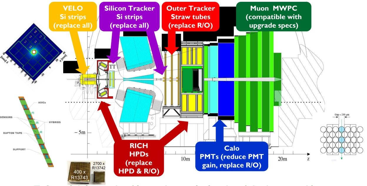
Completely new tracking system – pixel vertex detector, new strip
