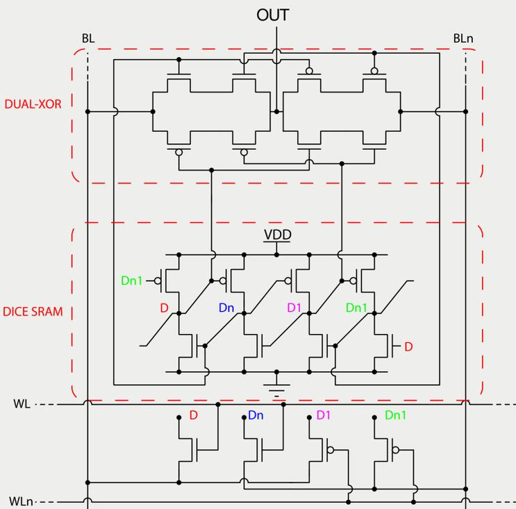
Schematic Diagram of the Radiation Hardened CAM
