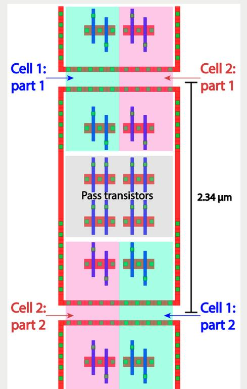
Interleaved layout of two Radiation Hardened CAM cells
