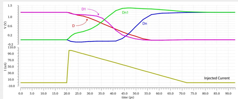
DICE simulation injecting 100 μA on Dn1 fall-time: 50 ps
