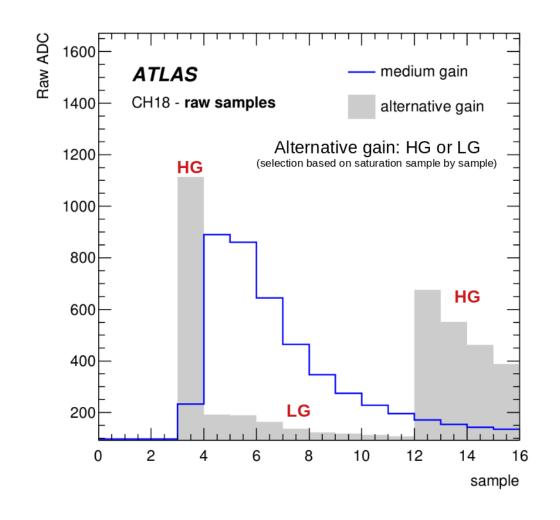
**Sample-by-sample gain selection** allows to output only the 2 gains which are relevant
