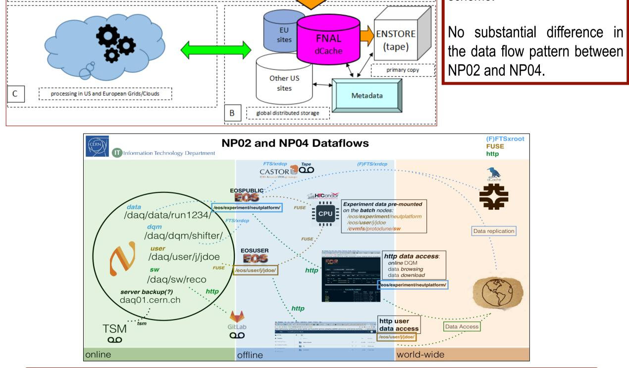
EOS serves as the staging area (for data quality monitoring and online/offline processing) from which the data gets committed to CASTOR (tape) and from which it is transmitted to a number of endpoints including principal data centers such as CERN Tier0, FNAL, IN2P3 and others.
