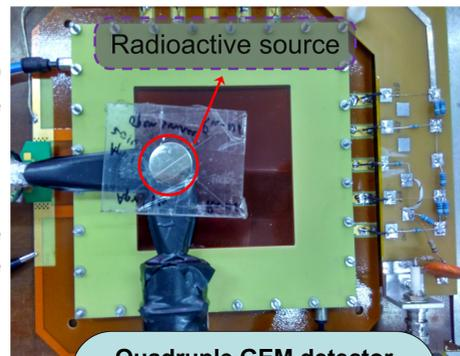
Quadruple GEM detector setup at VECC, Kolkata
