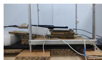
Figure 12: Cosmic ray test set up of both the MRPCs with three scintillators.
