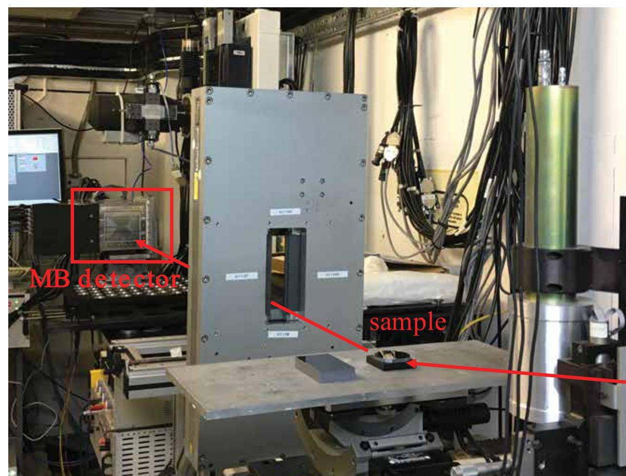
off-specular scattering from a Fe/Si neutron supermirror
