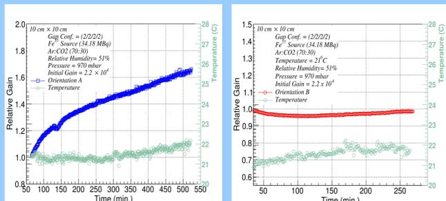
Fig. 15: Normalized gain as a function of time when the detector was continuously irradiated with source Fe-55. Gain increases in "Orientation A" upto 1.6 times the initial gain after the duration of around 8 hours while in "Orientation B" gain is almost flat. While, humidity, pressure and temperature were constant during the measurement but temperature has been added in the plot to demonstrate its stability.
