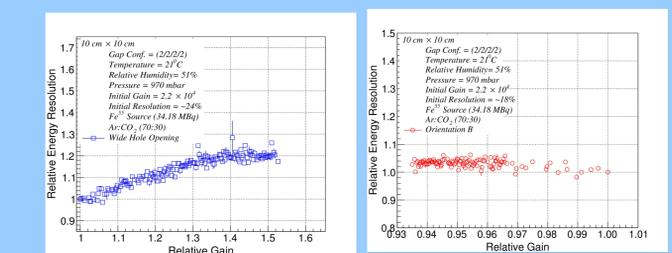
Fig. 19: The relative resolution measured as a function of relative gain when detector was continuously irradiated with Fe-55 source. The effect on energy resolution is clearly seen due to change in gain in "Orientation A" while as "Orientation B" doesn't appear to be much affected due to more stable gain.
