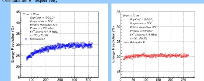
Fig. 18: Energy resolution measured as a function of time with the initial gain of  $2.2 \times 10^4$  when detector was continuously Fe-55 source. Resolution in "Orientation A" varies from  $\sim 24\%$  to  $\sim 30\%$ . The variation may be attributed to the change in gain as also shown in Fig. 20. On the other hand resolution in "Orientation B" is observed to show to less fluctuations and is almost flat at  $\sim 20\%$ .
