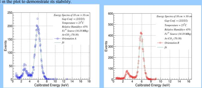
Fig. 16: The best values of the energy resolution  $\sim 23.71\% \pm 0.02$  and  $\sim 18.06\% \pm 0.01$  measured in "Orientation A" and in "Orientation B" with Fe-55 source. The resolution has been measured at a gain of  $2.2 \times 10^4$ .
