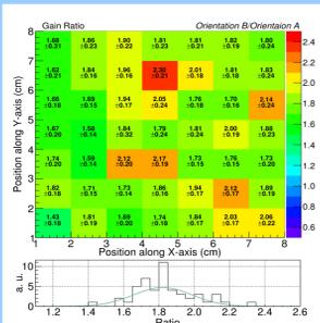
Fig. 14: Ratio of gains between "Orientation B" and "Orientation A" in each sector. The bottom histogram gives the mean value of the ratio of gains and is nearly equal to 1.8. The result demonstrates that the gain is 1.8 times higher in "Orientation B" compared to "Orientation A".
