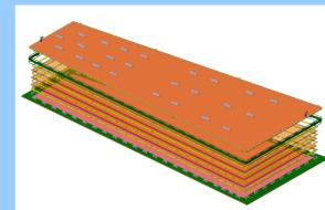
Fig. 7: Tripezoidal shaped GE1/1 detector to be used in CMS and the kind of large area GEM foils used in it
