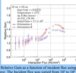
Fig. 21: Relative Gain as a function of incident flux using Ag target X-ray Source. The Incident flux was varied from  $10^2$  to  $10^6$  using copper attenuators of  $1 \text{ mm}$  thick, transparency increases till  $5 \times 10^4$  and after that a typical "bump" is observed (CMS region of interest  $< 10^4$ ). Similar result was reported to MPGD-2017 by CMS Muon Group and we confirm the result once again.
