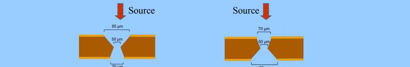
Fig. 8: Single-mask Single Asymmetric Holes: "Orientation A" (left) and "Orientation B" (right) facing the incident radiation.
