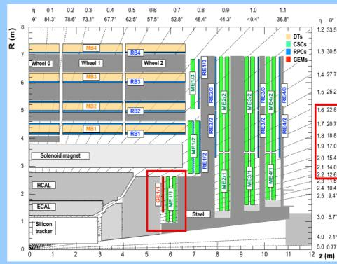
Fig. 1: A quadrant of the R-z cross-section of the CMS detector, highlighting in red the location of the GE1/1 station in the pseudo-rapidity region  $1.6 < |\eta| < 2.4$  [2]
