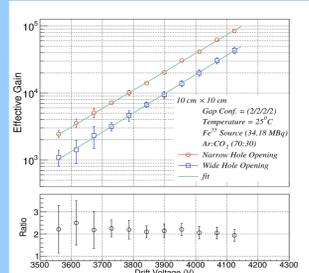
Fig. 12: Gain measured in a triple GEM  $10 \text{ cm} \times 10 \text{ cm}$  detector when all the three foils either with "Orientation A" or with "Orientation B" were facing the incident source (Fe-55). The ratio plot in the bottom shows that the gain almost 2 times higher in "Orientation B" compared to "Orientation A". Similar result has been presented at MPGD-2017 by CMS Muon Group and here we confirm the results once again.
