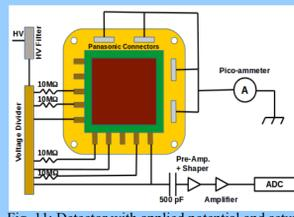
Fig. 9: Triple GEM Detector
