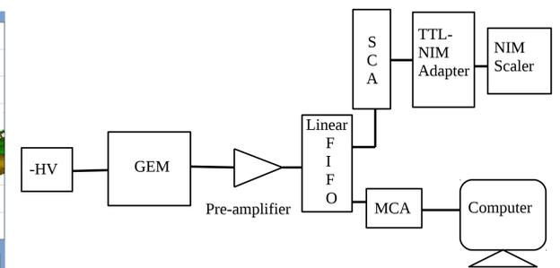
Schematic representation of the electronics setup
