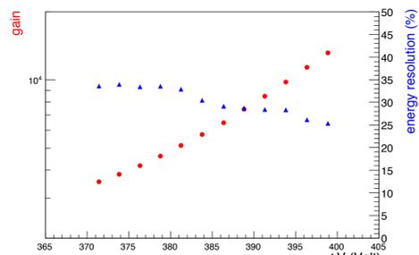
The gain and the energy resolution as a function of the GEM voltage. The error bars are smaller than the symbols.
