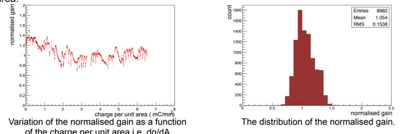
Variation of the normalised gain as a function of the charge per unit area i.e. dq/dA
