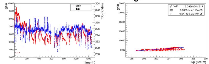
Variation of the measured gain and T/p as a function of the time.
