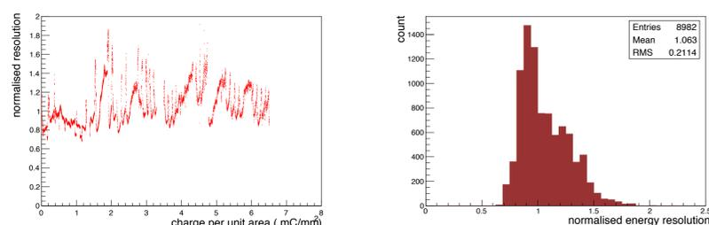
Normalised energy resolution as a function of the charge per unit area
