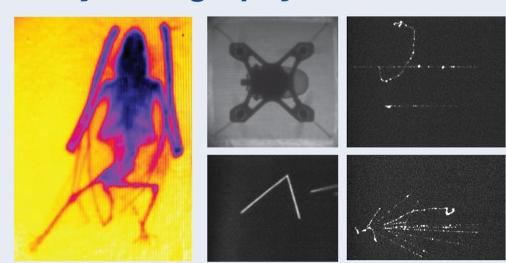
Optical read out of GEM-based detectors can be used for X-ray radiography and fluoroscopy as well as single event imaging. High gain factors permit sensitivity to radiation ranging from MIPs to highly ionising radiation.
