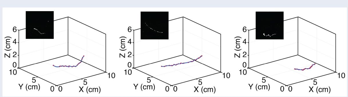
In addition to straight particle tracks like alpha particles, complex track geometries can be reconstructed by combining information from simultaneous electronic and optical readout. This permits the reconstruction of curved tracks as shown for cosmic events, which cannot be unambiguously visualised with timing information from a PMT. The combined readout approach thus extends the reconstruction capabilities of optically read out TPCs.
