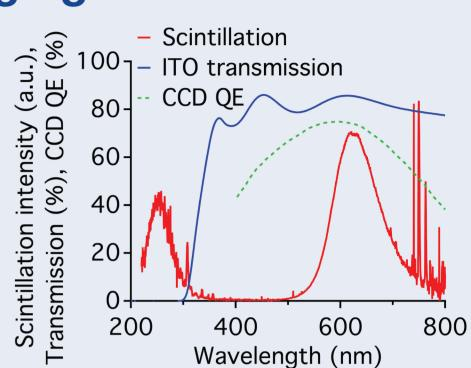
The emitted secondary scintillation light spectrum of Ar/CF<sub>4</sub> mixtures is compatible with the quantum efficiency (QE) of CCD imaging sensors and the transmission of ITO layers.
