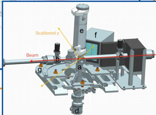
3D view of the characterization systems and its subsystems.
