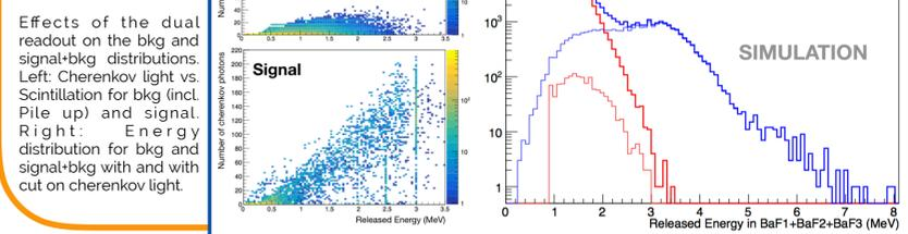
Effects of the dual readout on the bkg and signal+bkg distributions. Left: Cherenkov light vs. Scintillation for bkg (incl. Pile up) and signal. Right: Energy distribution for bkg and signal+bkg with and without cut on Cherenkov light.
