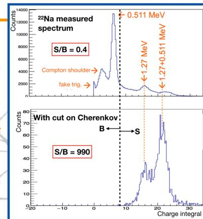
The rejection power of the dual readout technique has been tested with a <sup>22</sup>Na source.
