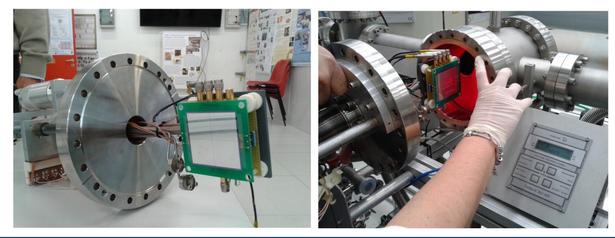
A standard sample (IAEA-C7 Oxalic Acid with certified radiocarbon concentration is  $49.53 \pm 0.12$  pMC) has been used to test the detector. A typical spectrum collected during the measurements for each sector are shown: the possible interferences are suppressed and only one peak is observed in the spectrum. From the integral under the signal is possible to retrieve the counting rate and also, thanks to a dedicated algorithm (work in progress) it will be possible to monitor the beam position.
