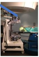
10+10 LFS + MPPC modules 2560 acq chns/head Distance from the isocenter=30 cm
