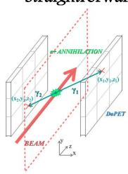
The annihilation position of each event is reconstructed by evaluating the intersection between the beam axis position provided by the TPS and the coincidence line detected by the scanner. Each coincidence event is weighted to take into account for its detection geometrical probability.
