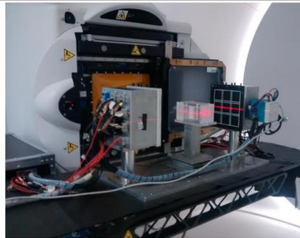
Figure 1. The DoPET system on the Trento treatment couch.
