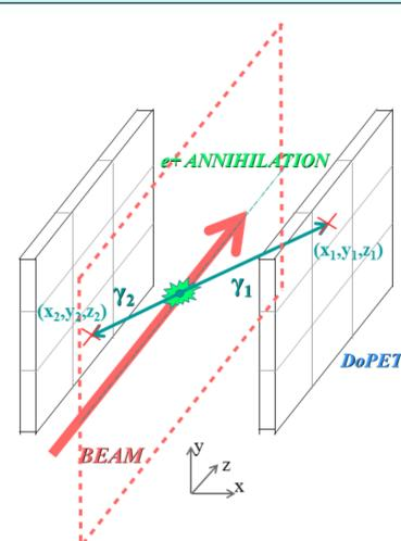
Figure 2. Sketch of the SFR reconstruction method
