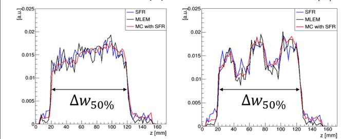
Figure 4. Reconstructed longitudinal profiles (beam axis). Data reconstructed with MLEM (black) and SFR (blue). The FLUKA prediction (red) reconstructed with SFR
