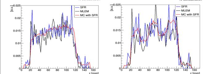
Figure 6. Longitudinal profiles corresponding to  $10^8$  primary protons. The zebra structure is not clearly recognizable anymore
