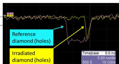
Fig. 9. alpha pulse waveforms before and after the first irradiation step
