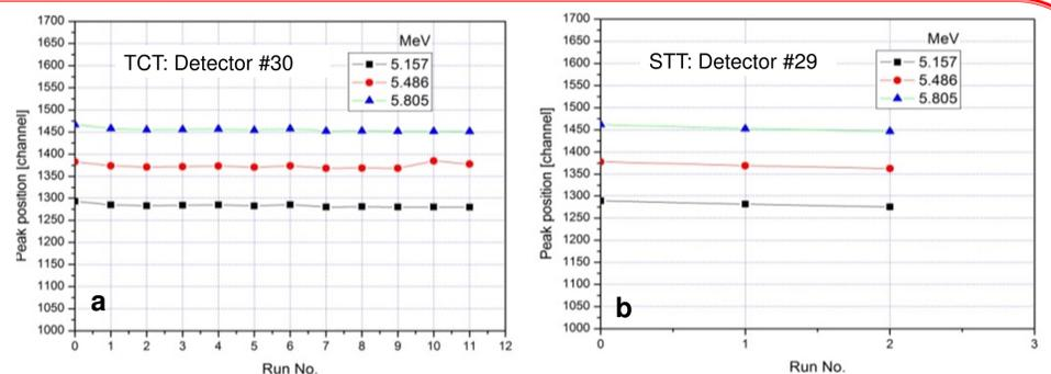
Fig. 5. Tri-alpha peak positions as function of run n. (time) in two weeks. (a) TCT; (b) STT
