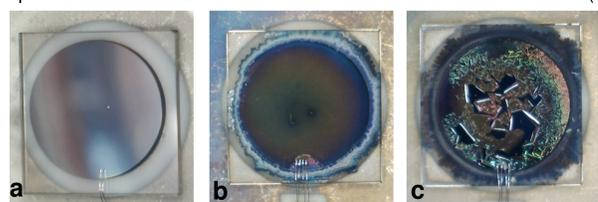
Fig. 6. sCD: (a) non irradiated; (b) 1.0 MGy; (c) 4.7 MGy.
