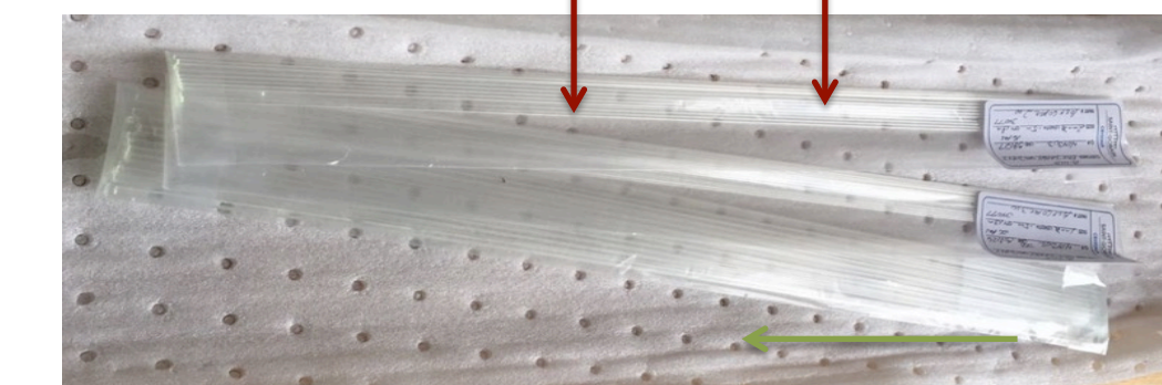
Scintillator Fibers, readout by photodiodes (not shown)
