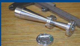
**Right:** one of the multi-mode horns to be mounted on the focal plane. The dismantled backshot shows the housing for the bolometer chip.
