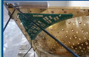
The **cold electronics** components are hosted on 8 boomerang-shaped PCBs to be mounted on the back of each quarter of the 2 focal planes. Each PCB hosts 3 readout chains of 18 channels, composed by a COG/NPO SMD capacitor and a superconducting inductor in series with each TES. Each chain is readout by a **6-series array SQUID** by VTT operated in a Flux Locked Loop (FLL) condition.
