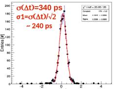
At: Time difference between two sensors reading the same crystal. Beam impact on crystal center
