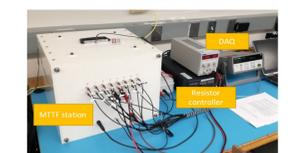
Test ensures MTTF >  $10^6$  hours for each batch.
