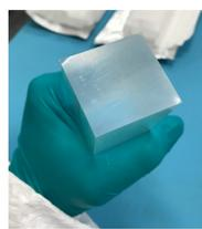
Reject crystals with dents, scratches or notches. Dimensional tolerance:  $\pm 100 \mu\text{m}$  Coordinate measuring machine (CMM) checks: transversal thickness, longitudinal length, face parallelism and perpendicularity
