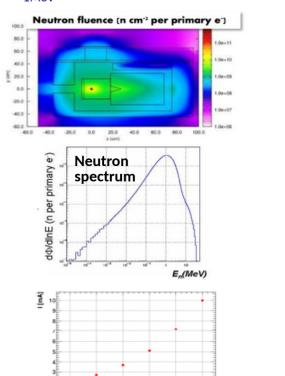
Dark current @  $20^\circ$  C after irradiation must be < 10 mA to ensure a current ~2 mA in the experiment
