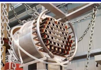
A calorimeter prototype (Module-0) has been built to validate the design. The module used crystal and SiPM preproduction samples tested for the international bid.
