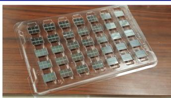
Hamamatsu devices have been selected after and international bid. Production is ongoing: 1 batch of 300 SiPM arrays/month Each of the 6 cells in the SiPM array is tested individually QA process will involve 24k cell characterizations! (1k performed as of May 2018).
