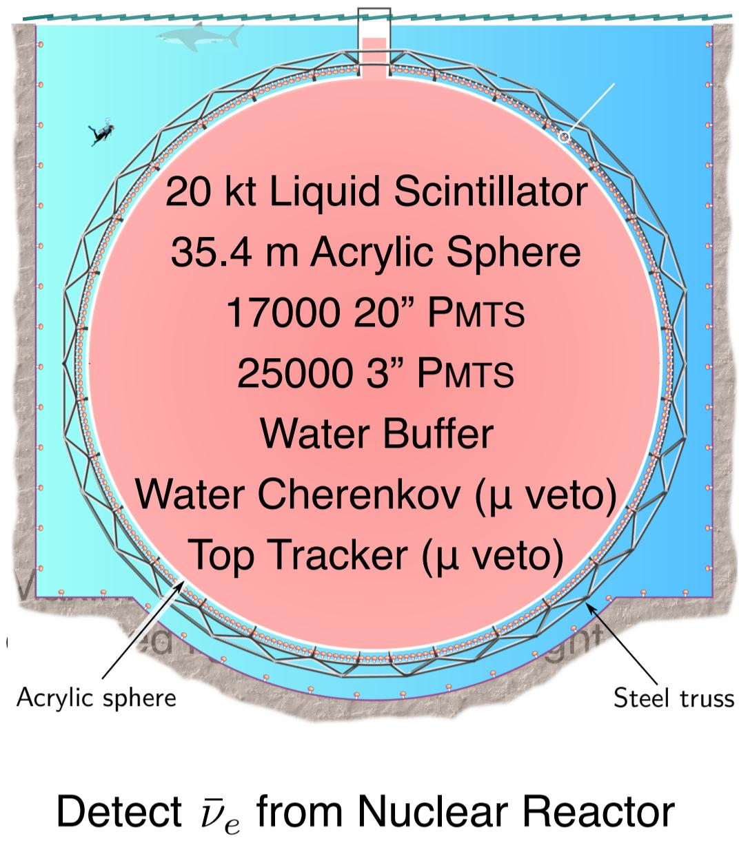
Goal: **Determine Neutrino Mass Ordering** by performing a precision measurement of the oscillated antineutrino energy spectrum at 53 km baseline
