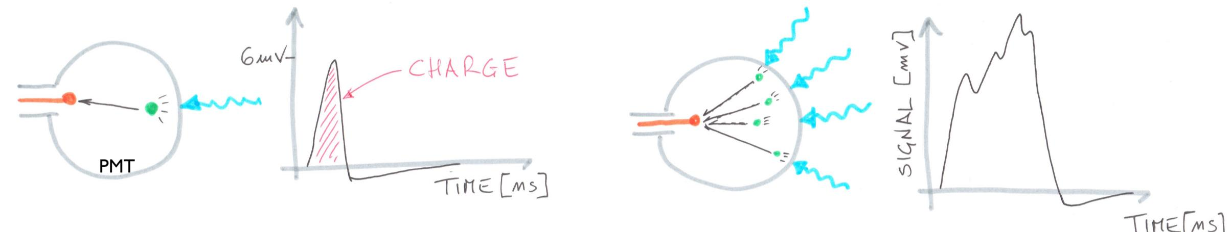
Detector response is nonuniform. Map it using calibration source (eg.  $^{60}\text{Co}$ )
