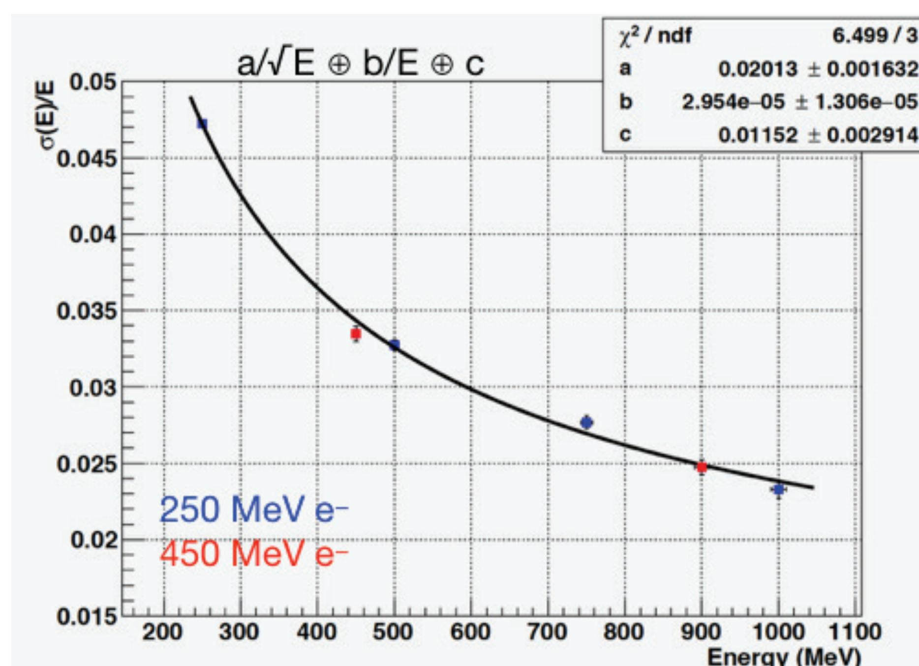
FIGURE 4. ENERGY RESOLUTION MEASURED WITH ECAL PROTOTYPE EXPOSED TO BTF ELECTRON BEAMS OF DIFFERENT ENERGIES
