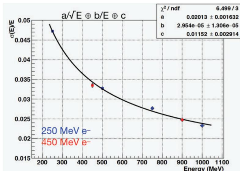
FIGURE 4. ENERGY RESOLUTION MEASURED WITH ECAL PROTOTYPE EXPOSED TO BTF ELECTRON BEAMS OF DIFFERENT ENERGIES
