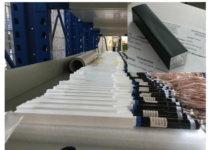
FIGURE 3. SCINTILLATING UNITS OF THE PADME ECAL. IN THE INSET ONE OF THE SAC CRYSTALS
