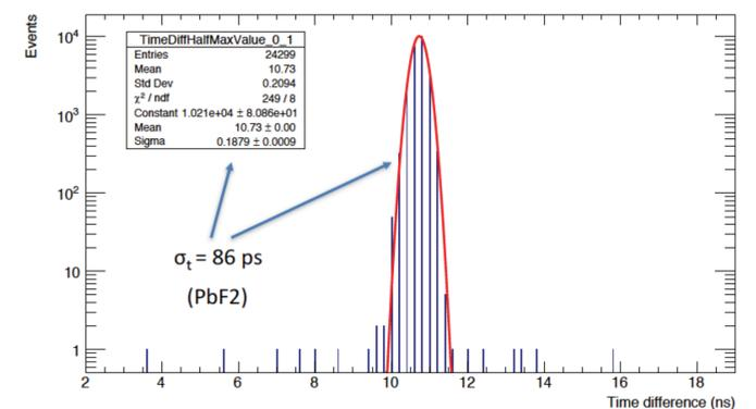
FIGURE 5. TIME RESOLUTION MEASURED WITH SAC PROTOTYPE
