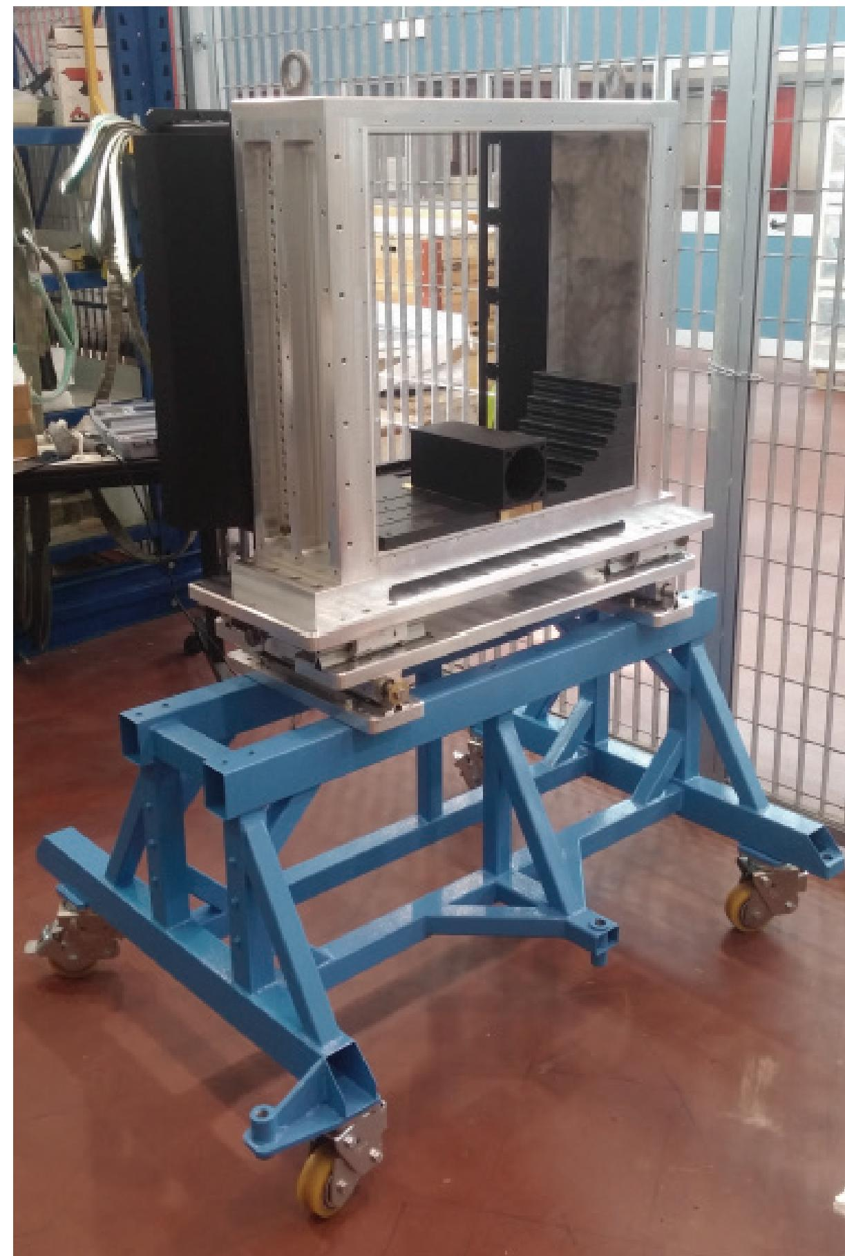
FIGURE 2. ECAL MECHANICAL STRUCTURE
